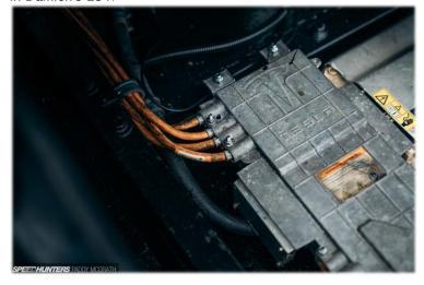
Getting the Tesla drive unit to communicate with a non-Tesla control system was one of the biggest challenges Damien faced. While he was able to take care of the hardware, he relied on the community at *OpenInverter.org* to assist with the software side. With the Tesla drive unit now under control, the next challenge was a more traditional 'engine swap' one — making the whole Tesla unit fit in the E31.
