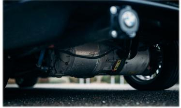
It was around this time that Damien acquired a Tesla Model S drive unit and things took a really interesting turn. The Tesla drive unit is an all-in-one package featuring the motor, inverter and differential, but is very much a 'closed shop' when it comes to communicating with non-Tesla control systems.
