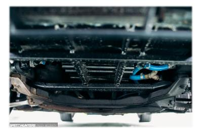
The next pieces of this new puzzle were the 16kWh batteries from a hybrid 2013 Vauxhall Ampera which were fitted at the front of the vehicle. They currently only offer around 80km (50mi) of range, but supply enough power to make the most of the Tesla drive unit, propelling the BMW from standstill to 60mph in around 3.4-seconds.
