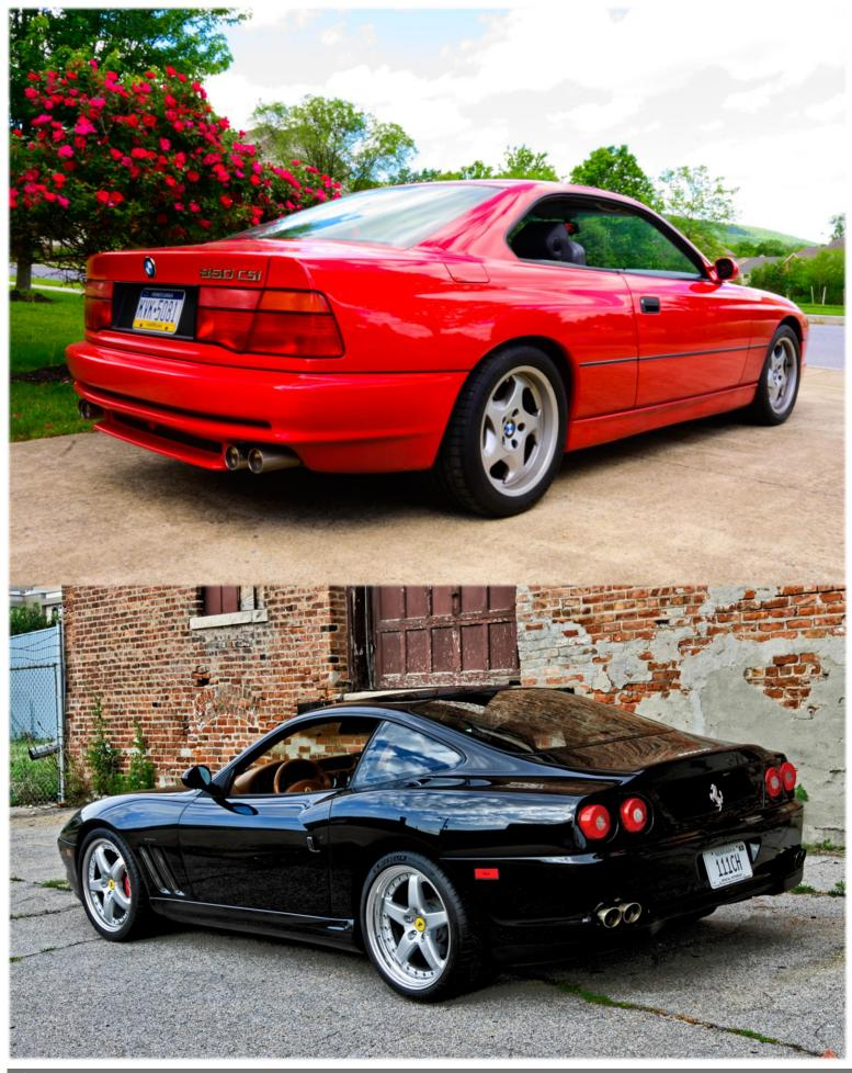
The top-of-the-range variant of the BMW E31 8 Series, the 850CSi was manufactured from 1992 to 1996, and featured a front-mounted engine, a six-speed manual transmission, and rearwheel drive with a 2.93:1 limited-slip differential. The CAD
